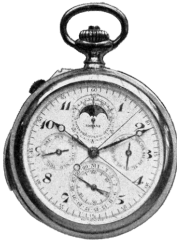
Fig. 125 – Dial of Triple Complicated Watch
