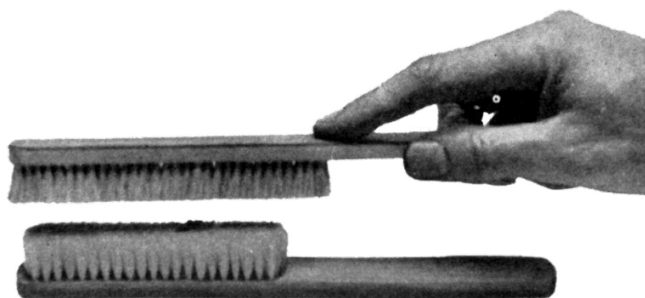
Fig. 126 – Method of Drying Small Components After Cleaning in Alcohol
