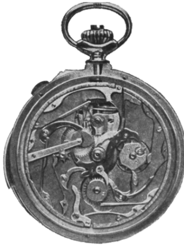
Fig. 124 – Showing Under Dial of Triple Complicated Watch
