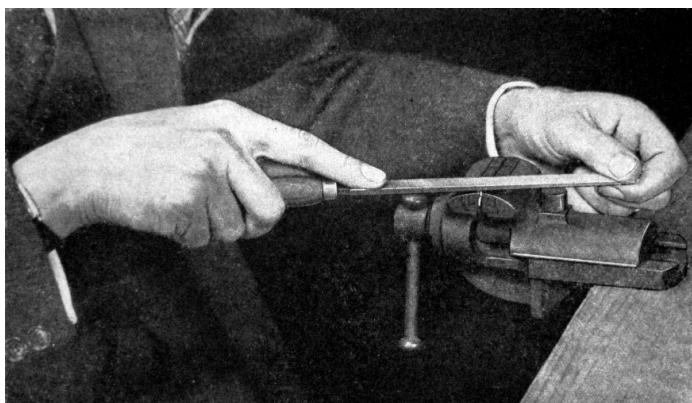
Fig. 2 – Using Large File
